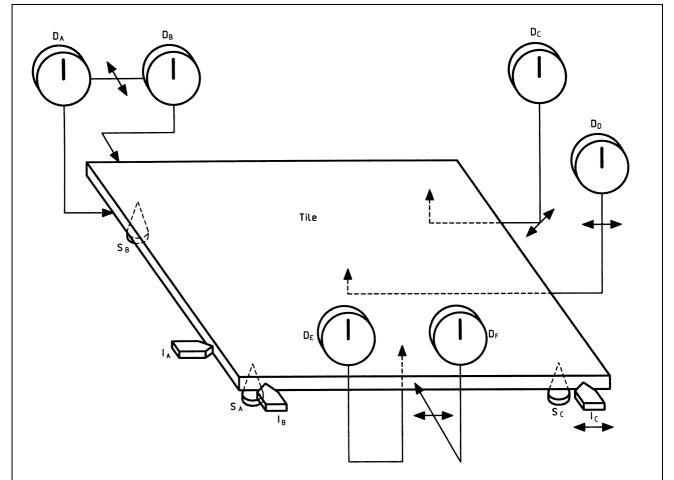
$\label{eq:Figure 1-Apparatus} Figure \ 1-Apparatus \ for \ the \ measurement \ of \ straightness \ of \ sides, \ rectangularity \ and \ surface \ flatness$
