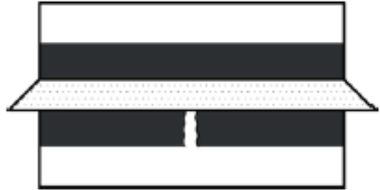
Stress Relief (for asphalt interlayer)
