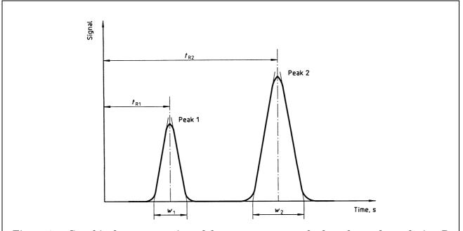
Figure 3 — Graphical representation of the parameters to calculate the peak resolution R
