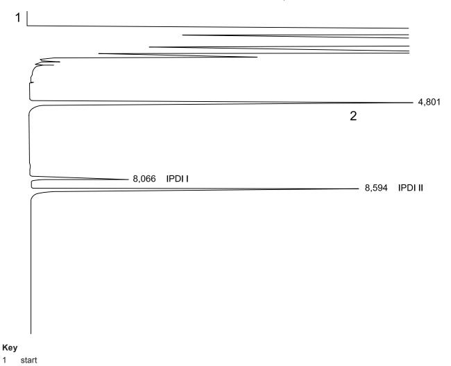
Figure 3 — Gas chromatogram for isophorone diisocyanate (second example)
