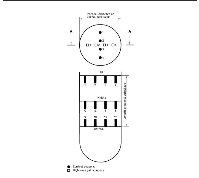
Figure 1 — Control coupon and high mass gain coupon positioning for establishing mass gain mean and standard deviation
