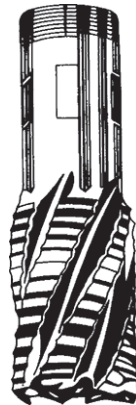
Figure C.3 — Chip-breaking mill cutter
