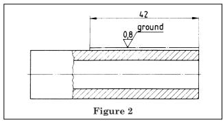
**5.2** Interchangeable conical or spherical ground joints complying with the requirements of ISO 383 and ISO 641 respectively, shall be designated in the manner described therein. Accordingly, no detailed dimensioning of that portion and no indication of the surface finish are required.
