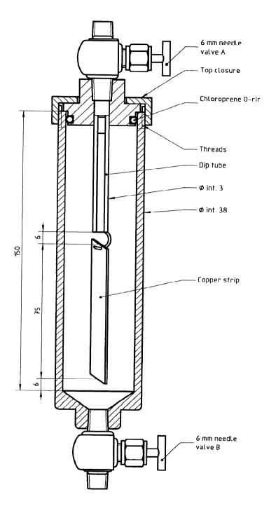
Material of test cylinder, dip tube, needle-valves: Stainless steel
