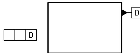
Figure C.1 — Plane — Input for reading (drawing indication) and for writing (design intent)
