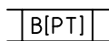
Figure 35 — Indication when only the point is needed in the set of situation features
