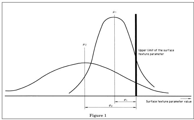
The reliability of the decision as to whether or not the surface being inspected meets the specification, and the precision of the mean value obtained for the surface texture parameter of the same surface, depend on the number of sampling lengths within the evaluation lengths with which the single value of the surface texture parameter is obtained and also on the number of evaluation lengths, i.e. the number of measurements along the surface.
