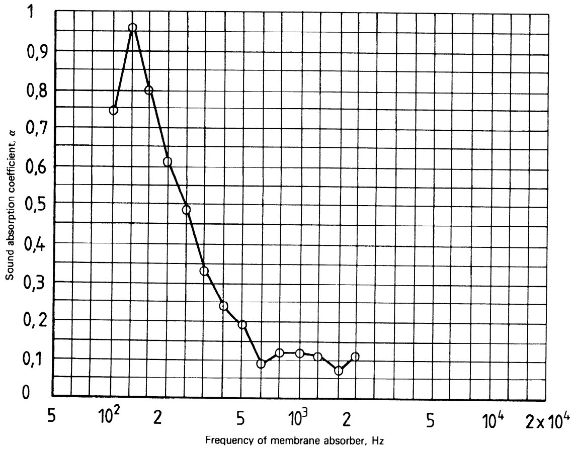
Figure B.2 — Sound absorption coefficient \alpha for the membrane absorber measured in a 200 m 3 reverberation room
