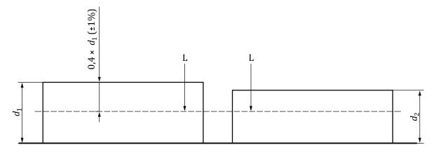
a) Test piece before fatigue test
