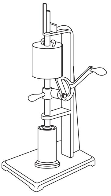
NOTE Each turn of the handle causes the weight to be raised and then dropped on the collar attached to the plunger shaft.
