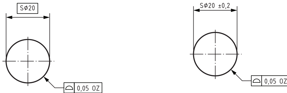
a) Surface profile specification for a sphere of defined nominal size, given by a TED with OZ indication
