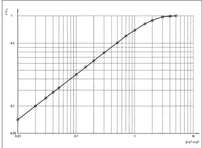
Figure A.1 — Water absorption  $c/c_s$  of sheets as a function of the dimensionless function D;  $^2 \cdot t/d_2$  (D = diffusion coefficient, t = immersion time, d = thickness of specimen)
