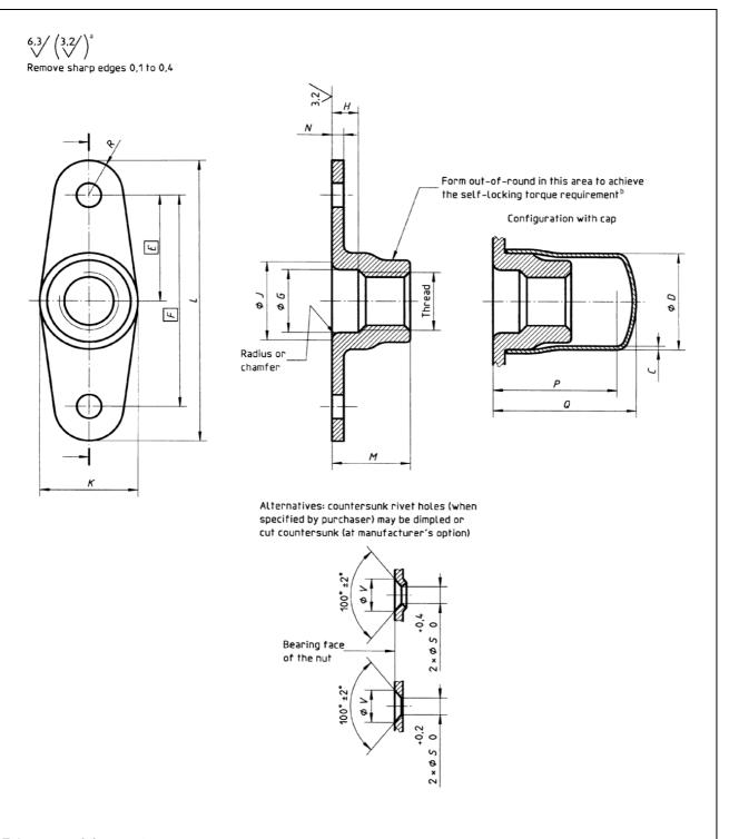
Tolerances of form and position shall conform to those specified in ISO 8788. Details of form not stated are at the manufacturer's discretion.
