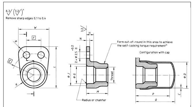
Tolerances of form and position shall conform to those specified in ISO 8788. Details of form not stated are at the manufacturer's discretion.
