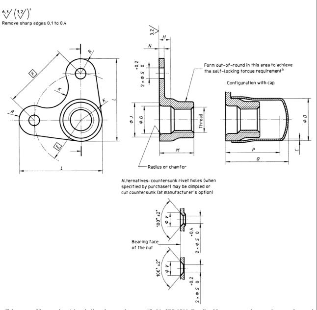
Tolerances of form and position shall conform to those specified in ISO 8788. Details of form not stated are at the manufacturer's discretion.
