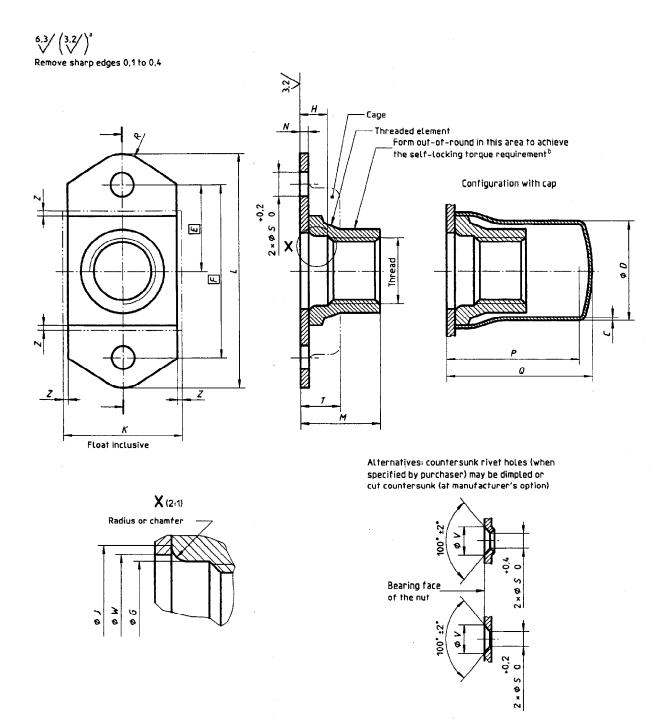
Tolerances of form and position shall conform to those specified in ISO 8788. Details of form not stated are at the manufacturer's discretion.
