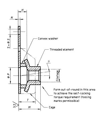
NOTE Tolerances of form and position shall conform to those specified in ISO 8788.
