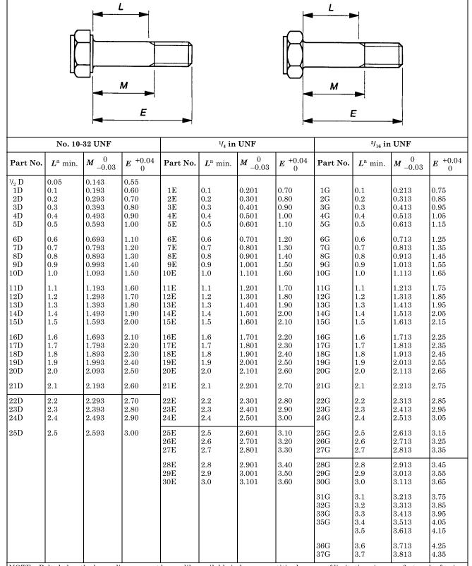
NOTE Bolts below the heavy line may not be readily available in large quantities because of limitations in manufacture by forging. <sup>a</sup> See **6.3**.
