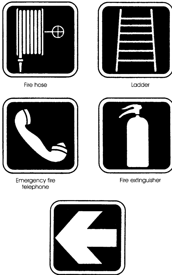
Figure 10.7 Fire-fighting equipment signs (red and white) specified in the Health and Safety (Safety Signs and Signals) Regulations
