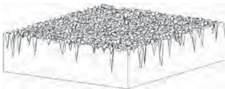
Fig. 20 —Generated non-Gaussian rough surface ( Sk=-1.75 , K=5.0 ).
