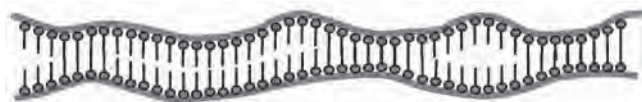
Fig. 2—Model of boundary lubrication proposed by Hardy, suggesting molecule adsorption in perfect order.
