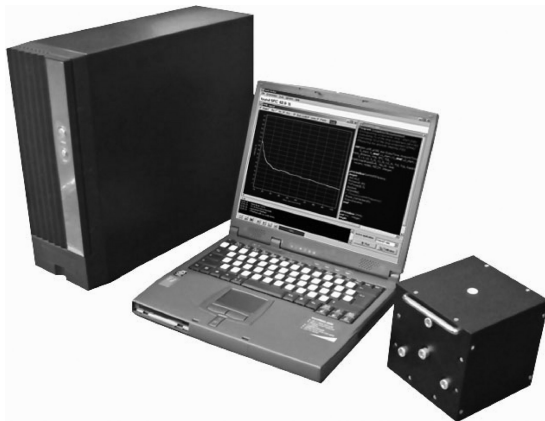
Fig. 1 —Typical TD-NMR Bench-top Spectrometer operating at 20 MHz, comprises a digital spectrometer (left), which is USB connected to a small computer. The 10-mm magnet system (right) weighs 8.5 kg and is 16 by 16 by 16 cm in dimension.
