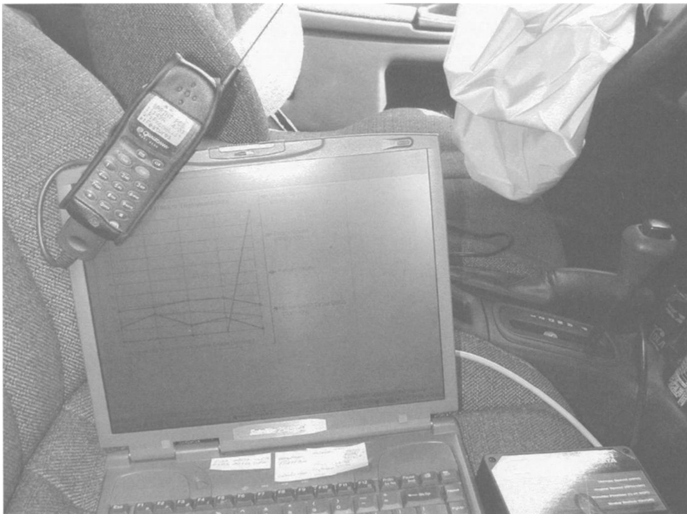
FIG. 3.25—A corollary feature of in-vehicle ECU EEPROM/flash memory downloads using laptop computers is that the data can be almost immediately uploaded via cell phone wireless data link to a laboratory for further analysis.
