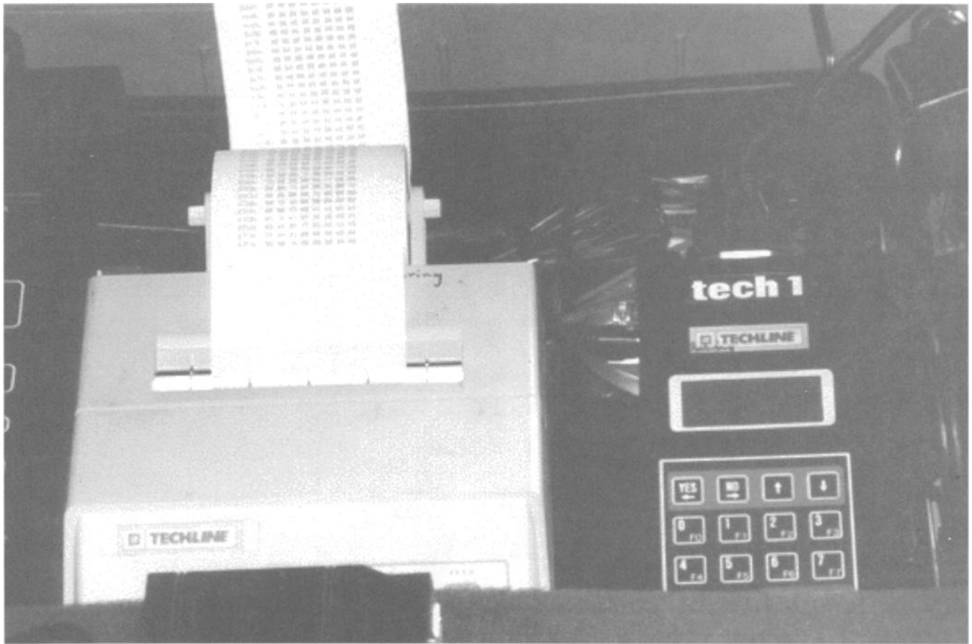
FIG. 3.18—Tech 1 scanner reading an SRS ECU and printing a paper tape with data and addresses in hex formatted list on paper tape.
