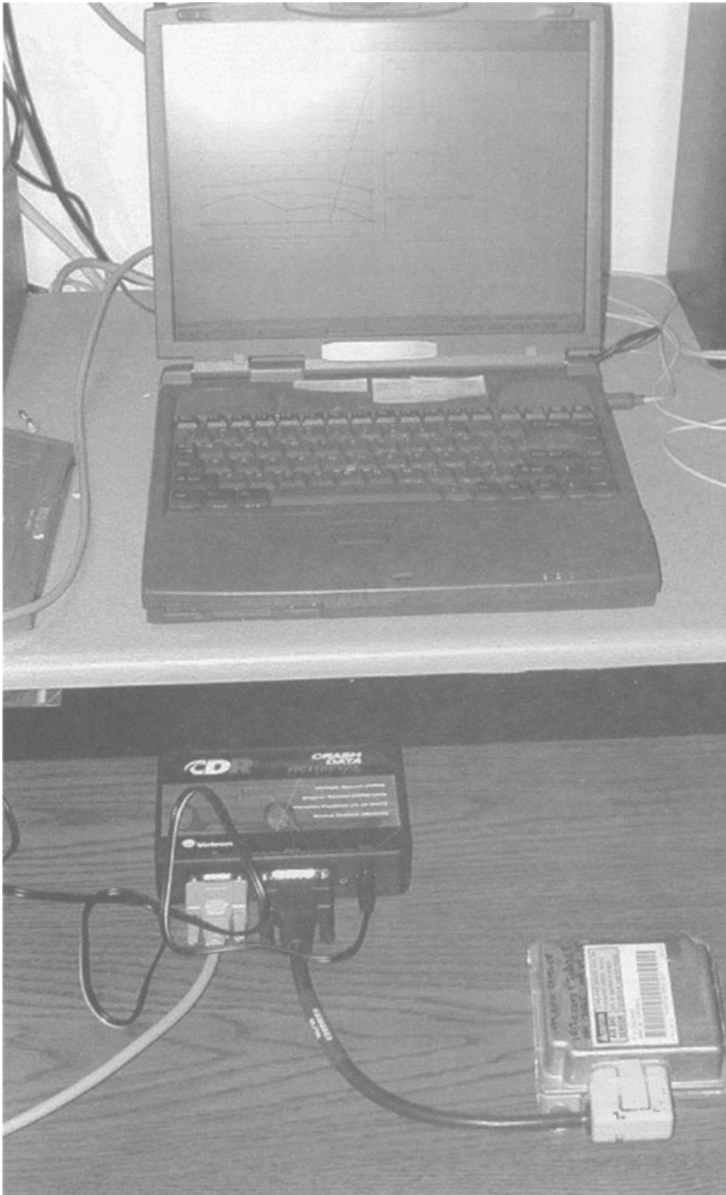
FIG. 3.26 —Benchtop interrogation of the 1999 domestic vehicle SRS ECU for crash data record in the, using laptop computer and Vetronix CDR interface. The data downloaded with the SRS ECU in and out of the vehicle was identical.
