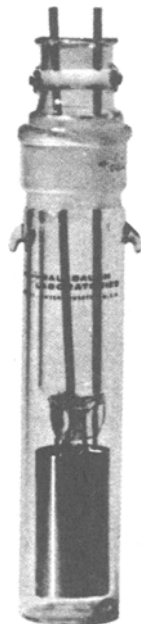
FIG. 1.70—Balsbaugh type 2TN50 two terminal concentric electrode cell.
