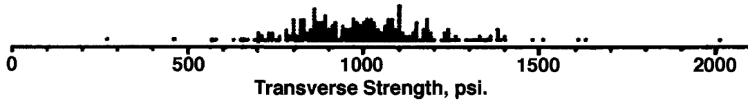
Fig. 2—Showing graphically the ungrouped frequency distribution of a set of observations. Each dot represents one brick, data of Table 2(a).
