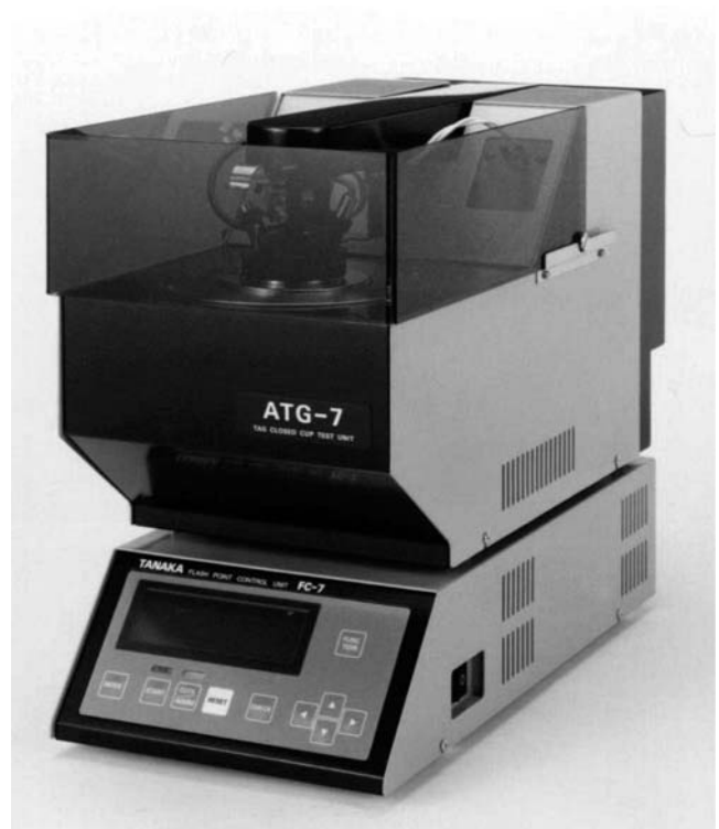
Figure 4.13—An example of an automated Tag closed-cup flash point apparatus. (Courtesy of Tanaka Scientific.)
