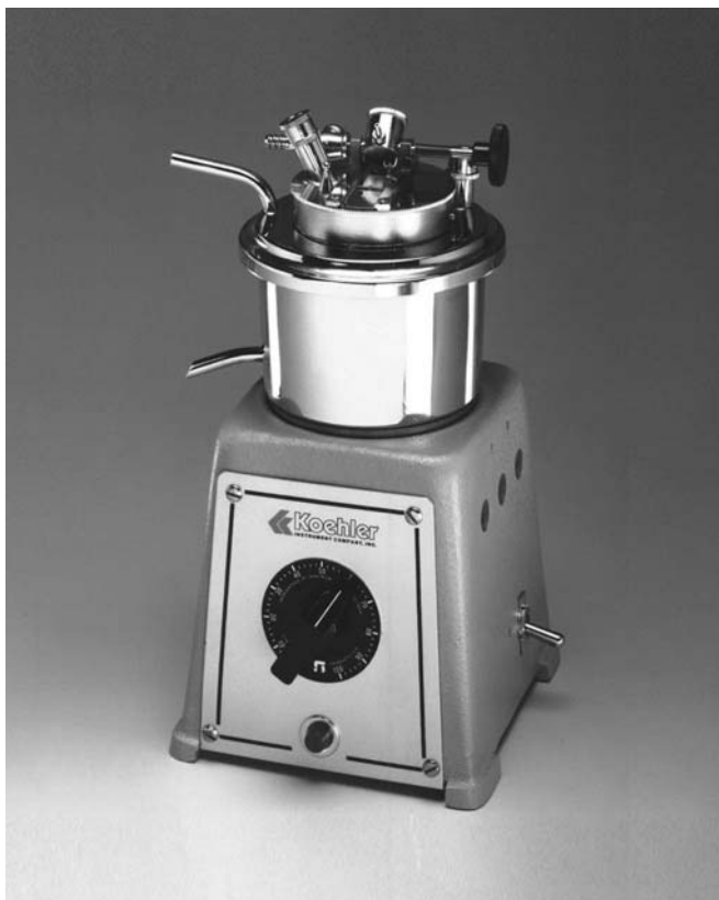
Figure 4.8 —An example of a manual Tag closed-cup flash point apparatus. (Courtesy of Koehler Instruments.)
