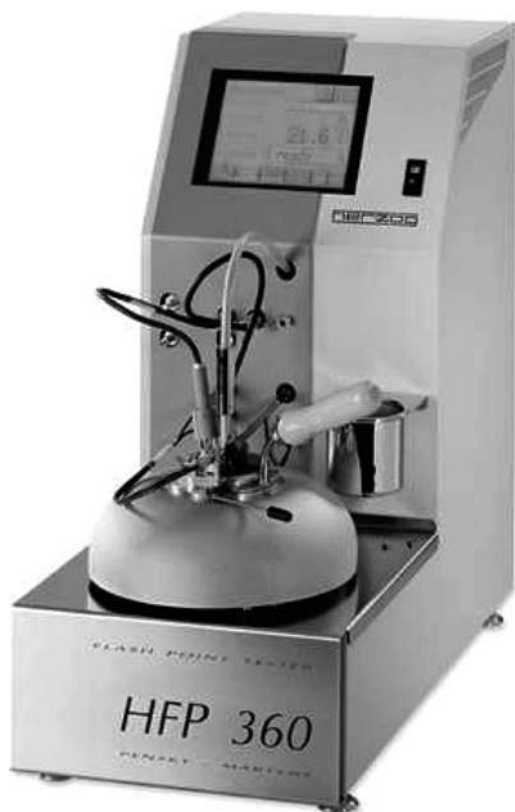
Figure 4.14 —An example of an automated Pensky-Martens closed-cup tester. (Courtesy of Petroleum Analyzer Corporation.)
