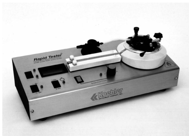
Figure 4.16—An example of a manual small-scale closed-cup tester. (Courtesy of Koehler Instruments.)
