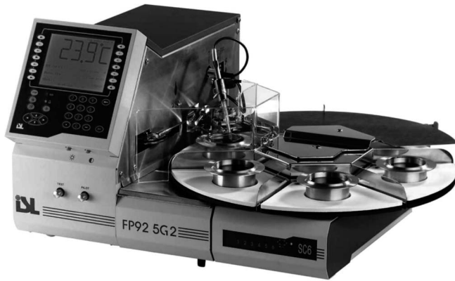
Figure 4.20 —An example of a flash point instrument with an automatic sample changer. (Courtesy of Petroleum Analyzer Corporation.)
