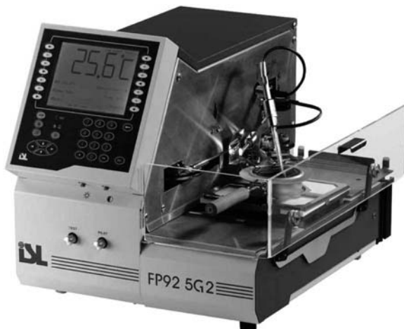
Figure 4.11—An example of an automated Cleveland open-cup flash point apparatus. (Courtesy of Petroleum Analyzer Corp.)
