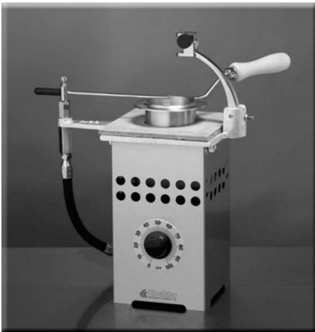
Figure 4.2—An example of a manual Cleveland open-cup flash point apparatus. (Courtesy of Koehler Instruments.)
