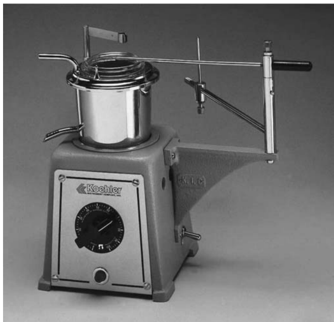
Figure 4.4 —An example of a manual Tag open-cup flash point apparatus. (Courtesy of Koehler Instruments.)
