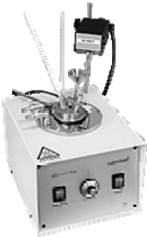
Figure 4.6 —An example of a manual closed-cup Abel flash point tester. (Courtesy of Petrotest Instruments.)
