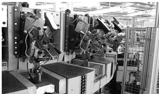
FIG. 1.7 Direct attach process. (With permission from the Desma Shoe Machine Company, available at www.desma.de .)
