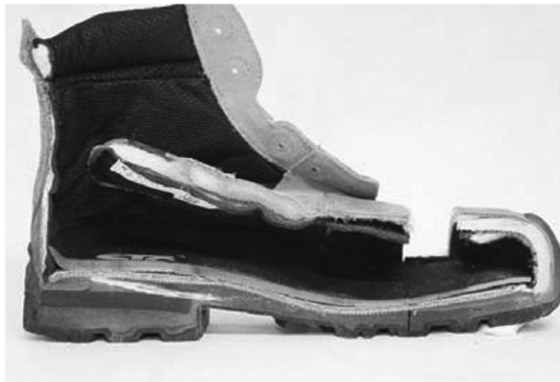
FIG. 4.8 Integrated puncture-resistant device. Boot for testing courtesy of STC Footwear ( www.stcfootwear.com ). (With permission from Precision Testing Laboratories, available at www.precisiontesting.com .)
