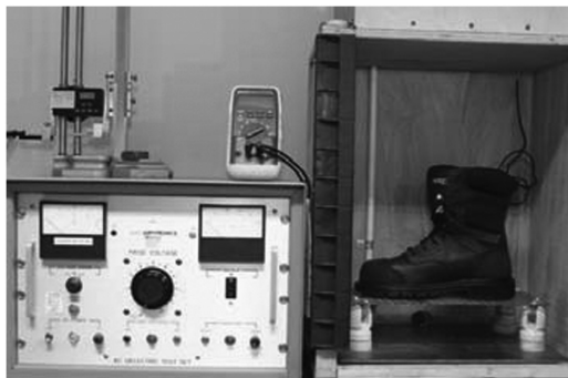
FIG. 4.5 Electrical hazard testing. (With permission from Precision Testing Laboratories, available at www.precisiontesting.com .)
