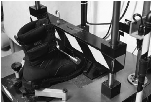
FIG. 4.3 Metatarsal impact testing. (With permission from Precision Testing Laboratories, available at www.precisiontesting.com .)
