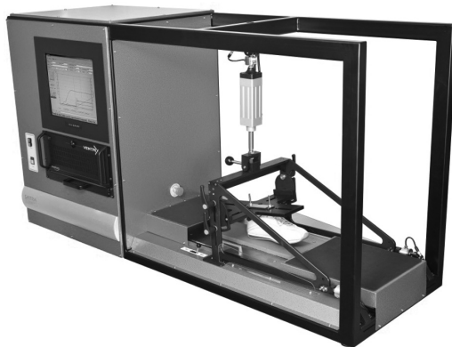
FIG. 5.13 SATRA STM 603 whole shoe tester. (With permission from SATRA Technology Centre, Kettering, Northants, United Kingdom, available at www.satratechnology.com .)
