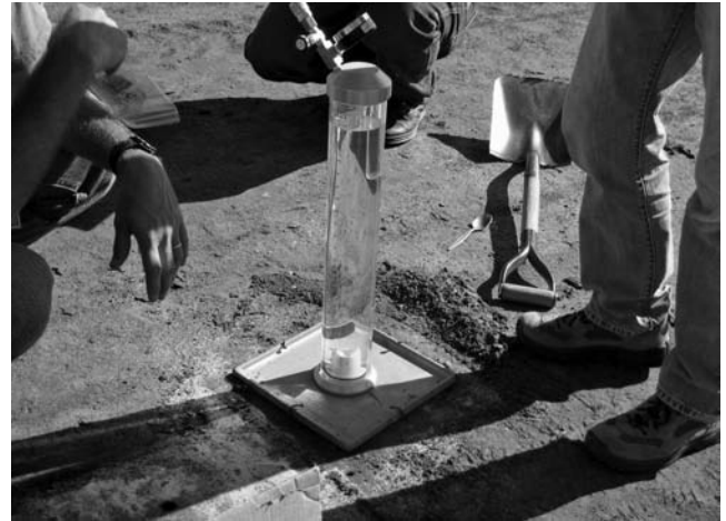
Fig. 6C—Rubber balloon method (ASTM D2167).
