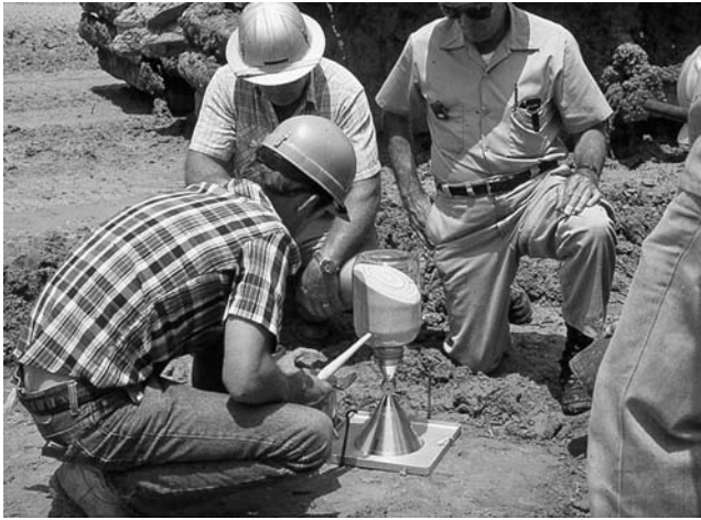
Fig. 5C—Sand cone method (ASTM D1556).
