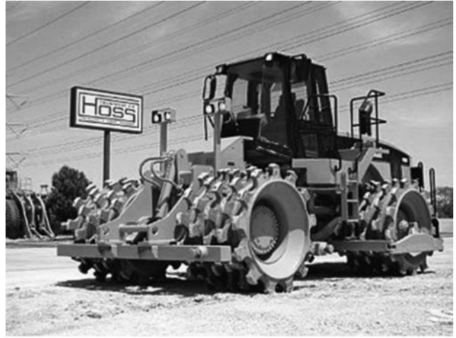
Fig. 2C —Self-propelled tamping roller—provides the same kneading action for plastic soils.
