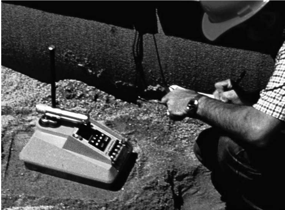
Fig. 9C—Nuclear method (ASTM D6938).
