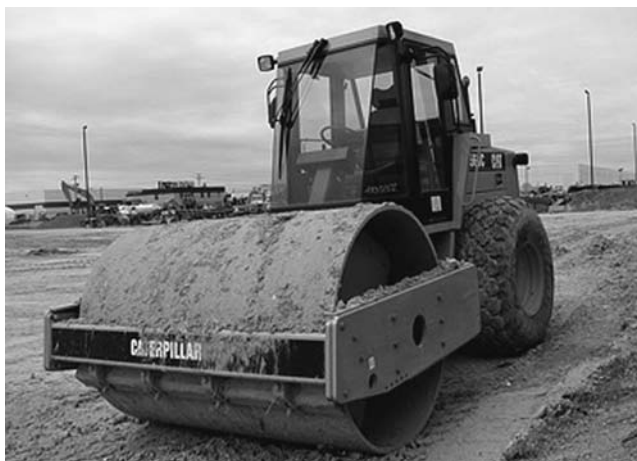
Fig. 12—Smooth wheel by static pressure and/or vibration as needed.
