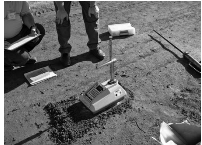
Fig. 8C—Nuclear method (ASTM D6938)
