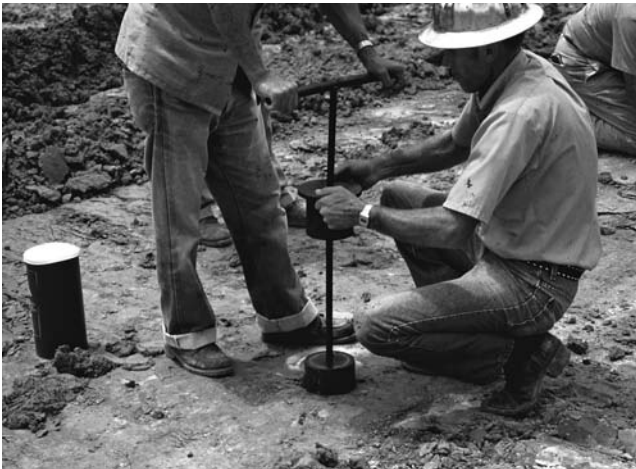
Fig. 7C—Drive cylinder method (ASTM D2937).
