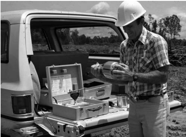
Fig. 10C—Calcium carbide gas pressure tester method (ASTM D4944).
