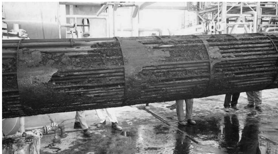
Fig. 11—Refinery heat exchanger fouled by asphaltenes (Courtesy of Professor G. A. Mansoori).
