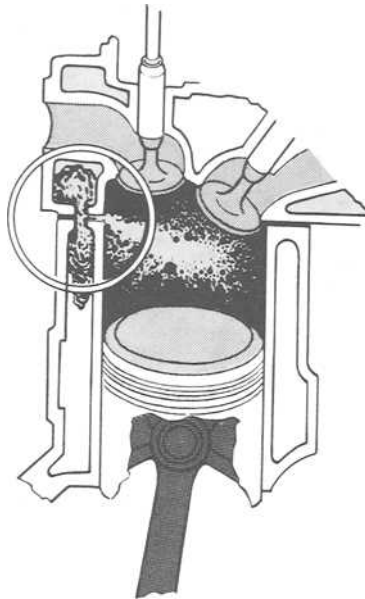
FIG. 3—Exhaust gas leakage into the cooling system can cause foaming, overflow, loss of coolant, overheating, and shortened inhibitor life with subsequent corrosion and rust clogging.
