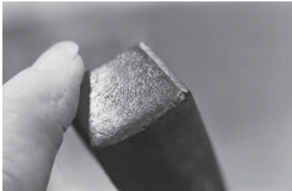
Fig. 9-15—Surface fatigue on a hammer head (as the result of repetitive impact).
