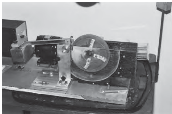
Fig. 10-8—ASTM B 611 high-stress abrasion test for cemented carbides.
