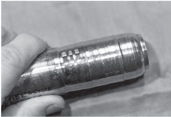
Fig. 1-6—Pump sleeve abraded by contaminants in packing.
