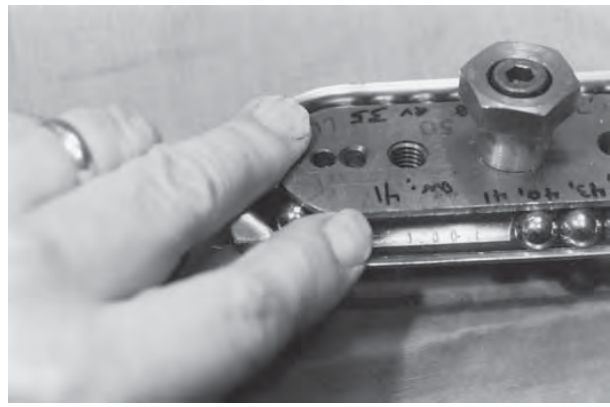
Fig. 9-8—False brinelling (from microscopic oscillatory motion of the bearing balls).
