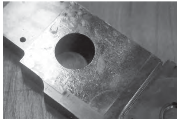
Fig. 8-16—Typical “gnarled” surface from fretting (420 stainless-steel injection mold part; hole is 35 mm in diameter).
