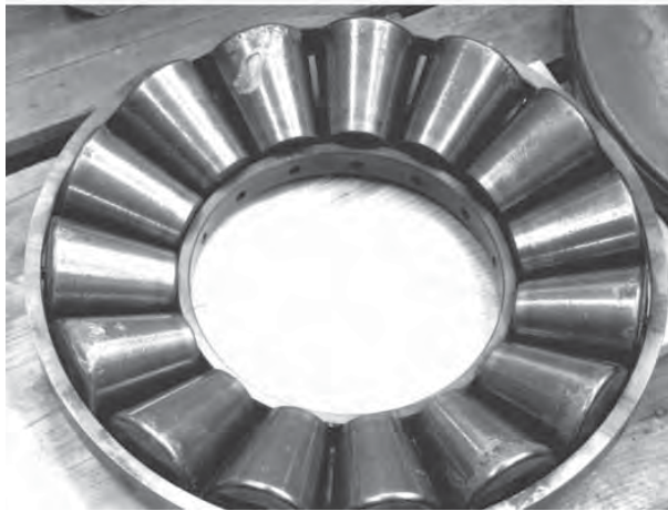
Fig. 1-14—Surface fatigue of a million-pound thrust bearing.
