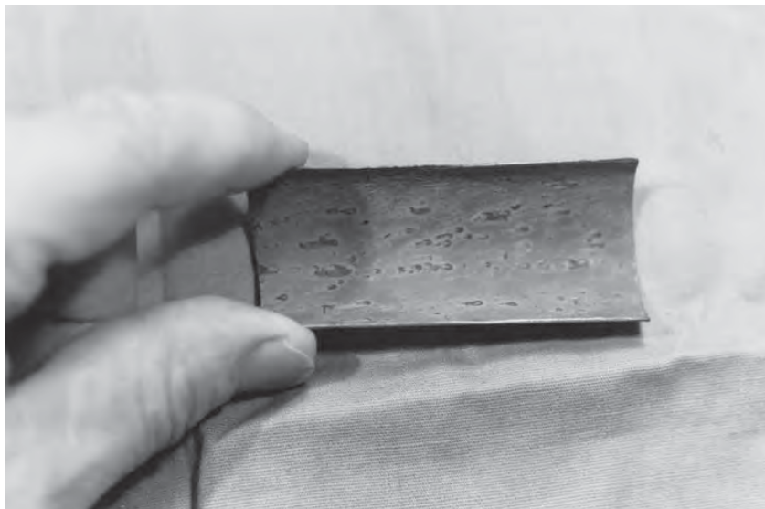
Fig. 1-26—Impingement erosion on the inside of a copper water pipe.
