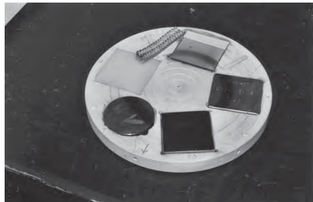
Fig. 10-13—Erosion of corrosion resistance materials after 30-day rub test versus rubber belting.
