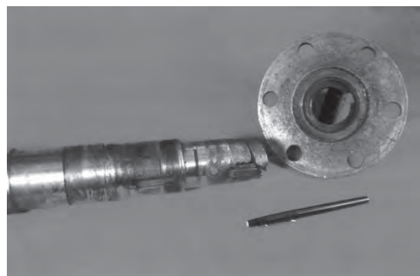
Fig. 5-12—Example of oxidative wear (near threads).
