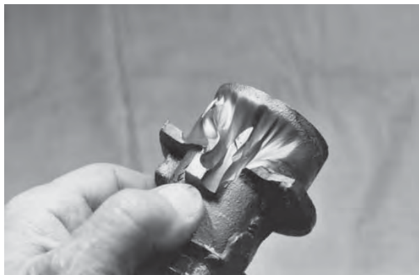
Fig. 1-22—Solid particle erosion of a sand blast fitting.
