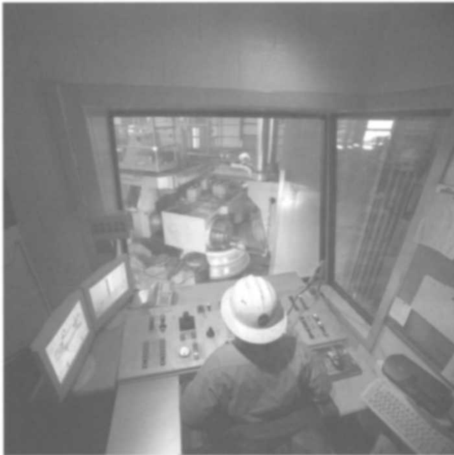
Fig. 5.11 —Examples of large ring rolling machines. The upper picture shows a mill capable of producing rings with an OD up to 23 ft (7 m). The radial power is 800 tons (725 t) and the axial power 500 tons (45 t). The lower picture taken from the control room of a modern ring rolling mill gives an impression of how such operations economize on manpower. In this example the maximum radial power is 1000 tons (907 t) and the axial power is 500 tons (45 t). A tapered gear ring is being forged. (Courtesy SMS Eumuco Wagner Banning, Witten, Germany)
