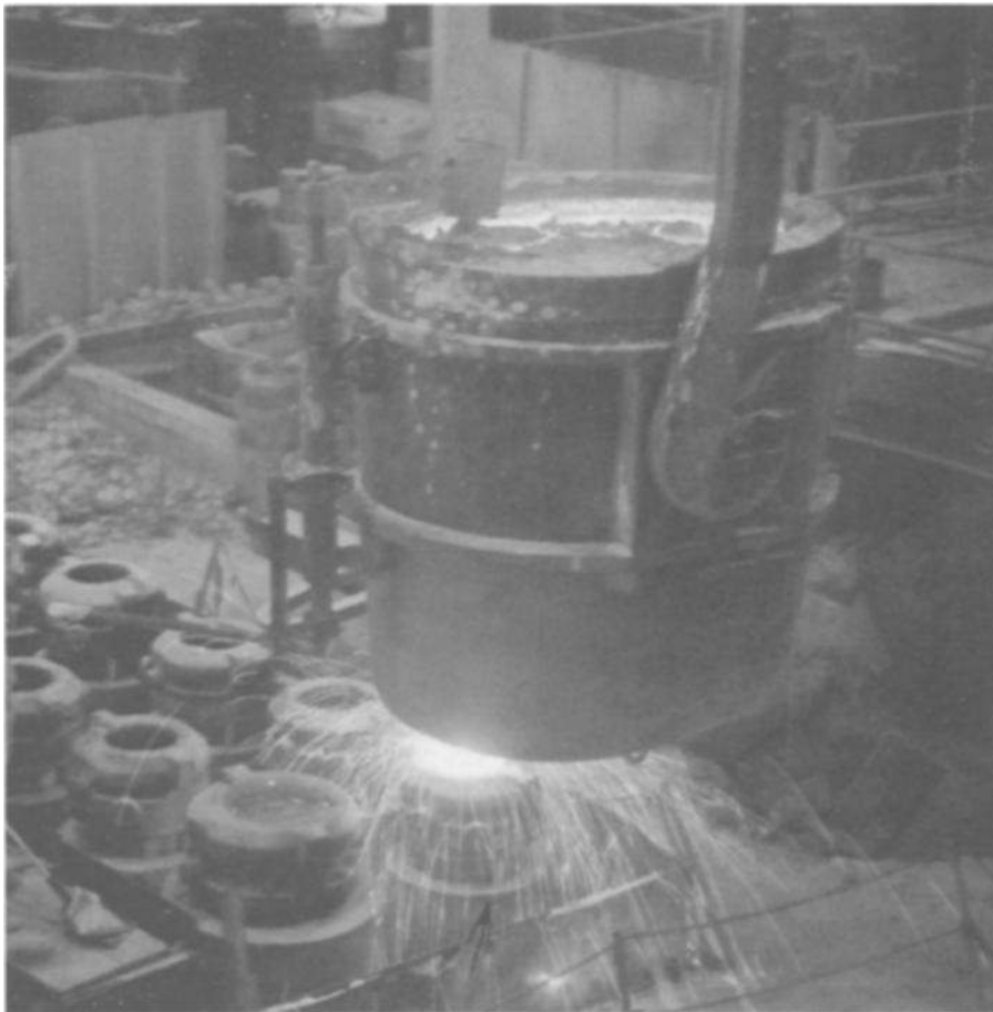
Fig. 13.1 —Forging ingots being top poured. The ingot to the front left foreground has been teemed and the hot top supports removed. The wooden supports are fitted between the cast iron hot top case and the top of the ingot mold before teeming begins. These maintain the hot top position until the mold has been filled, but must be removed immediately afterwards to permit the hot top to settle.
