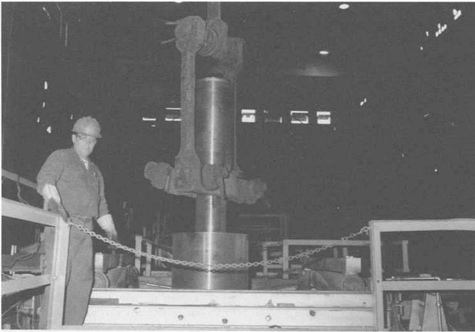
Fig. 9.4 —Hot rigging, of the type sometimes used in the heat treatment of rotor forgings. Although this particular system would not permit the forging to be rotated during air cooling, this forging was to be water quenched. The forging is being loaded into a vertical furnace through the split cast steel door. This runs on wheels that can be seen in the foreground.
