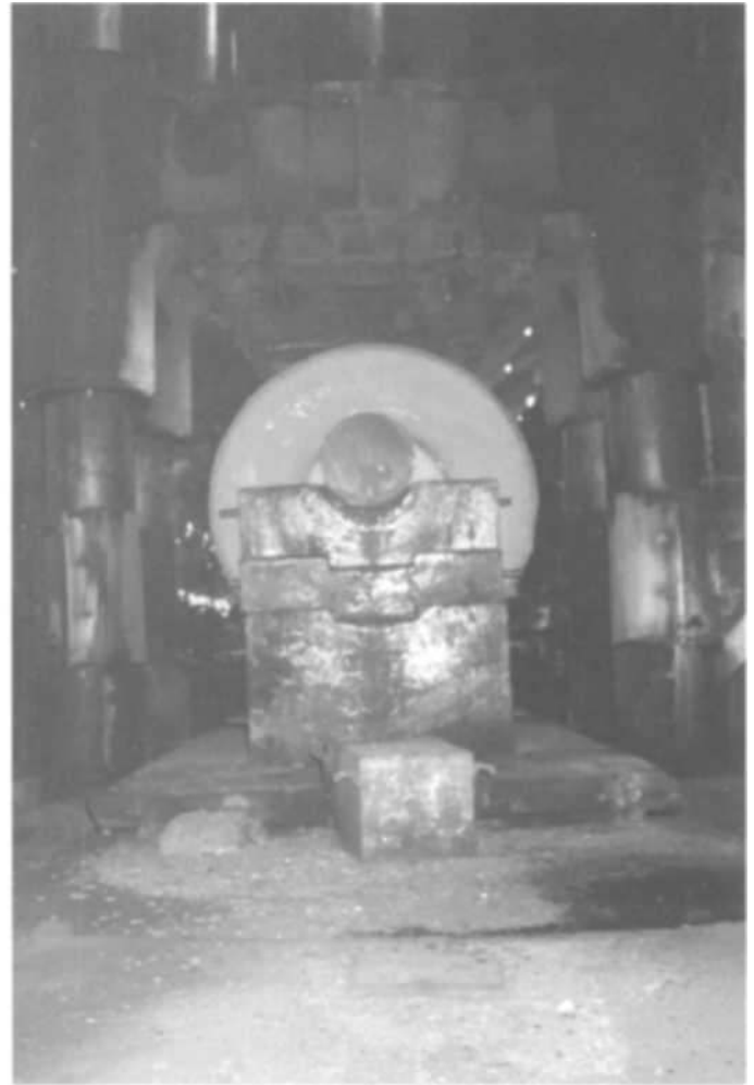
Fig. 5.4 —Once bored, the upset forging can be expanded on an open die press by forging between a special axially oriented top die and a mandrel bar that rests on supports at each end of the forging. The bottom press die does not come into play and is moved out of the way. The forging is rotated during this operation in which the axial length remains constant, but the diameter increases and the forging wall thickness is reduced. (Courtesy of The Japan Steel Works, Ltd.)
