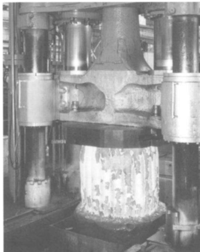
Fig. 2.1—Upset forging, compressing the ingot to reduce the axial length and increase the diameter. The length after upsetting is typically half of the initial length. (Courtesy A. Finkl and Sons Company)
