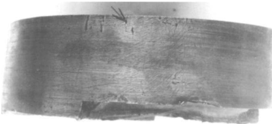
Fig. 21.4 —Failed cement kiln shaft forging. Failure was by fatigue originating at bronze grain boundary penetration stemming from an earlier bearing seizure. The shaft surface had been cleaned but particles of bronze could still be seen. Notice the alignment of the fracture path with the circumferential scores that were sites of bronze penetration.
