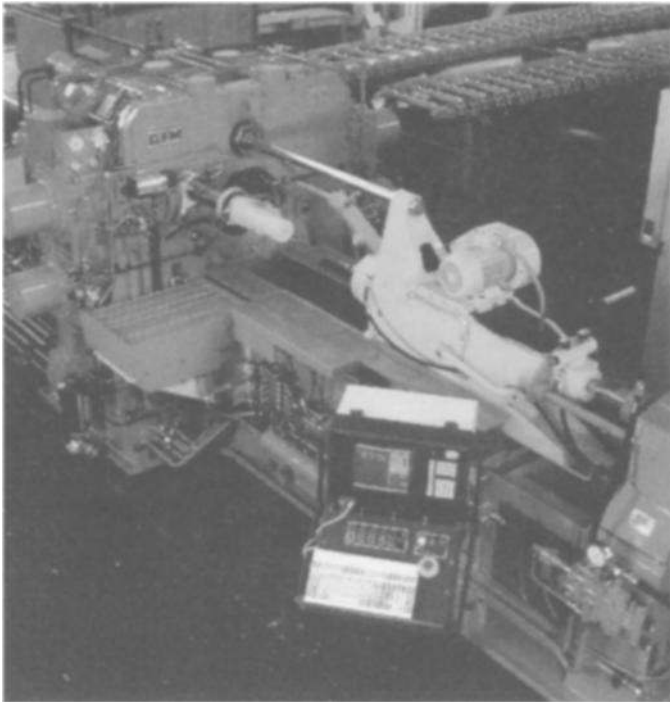
Fig. 5.7—Typical radial rotary forging machine in operation. The feed stock could be as-cast billets, wrought bar, or bored performs. (Courtesy American GFM Corporation)
