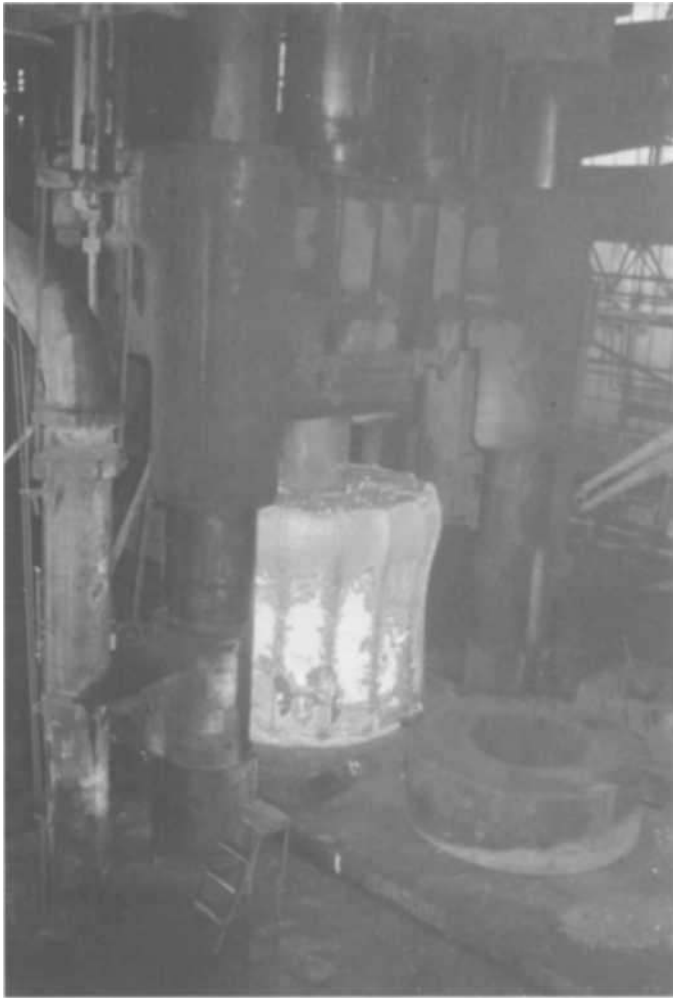
Fig. 5.3 —Hot trepanning the upset forging removes the segregated central core, a preparatory step to forging over a mandrel to expand the bore, or to reduce the wall thickness and increase the length of the forging. (Courtesy of The Japan Steel Works, Ltd.)
