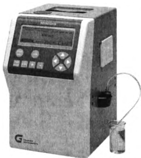
Fig. 11 —An example of a mini distillation instrument. (Images courtesy of Grabner Instruments.)
