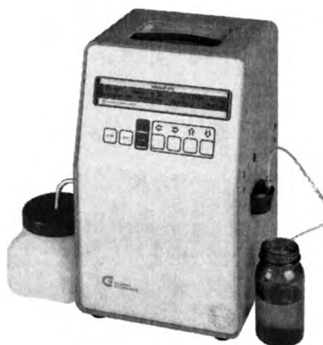
Fig. 4—An example of an automatic vapor pressure instrument for D5191. (Used with permission from Grabner Instruments).
