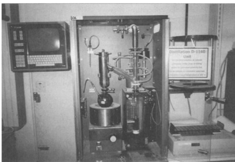
FIG. 3.7—An apparatus for experimental measurement of boiling point at reduced pressures by ASTM D 1160 test method (courtesy of KISR).
