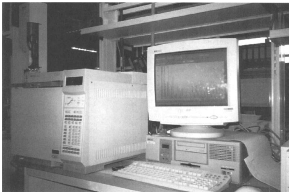
FIG. 4.2—A GC for measuring SCN distribution in crude oils and reservoir fluids (courtesy of KISR [5]).
