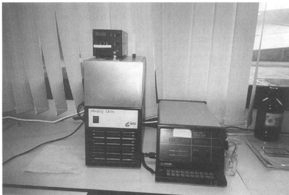
FIG. 3.8—PARA model DMA 48 digital density meter (courtesy of Chemical Engineering Department at Kuwait University).
