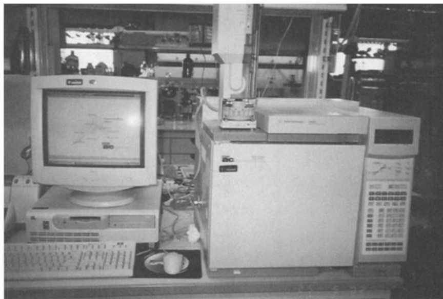
FIG. 3.6—A GC for measurement of boiling point of products (courtesy of KISR).
