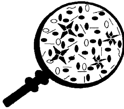
(a) Colloidal Phenomenon Due to Increase in Concentration of Polar Miscible Solvent (such as polar aromatic hydrocarbons shown by solid ellipses) in crude oil
