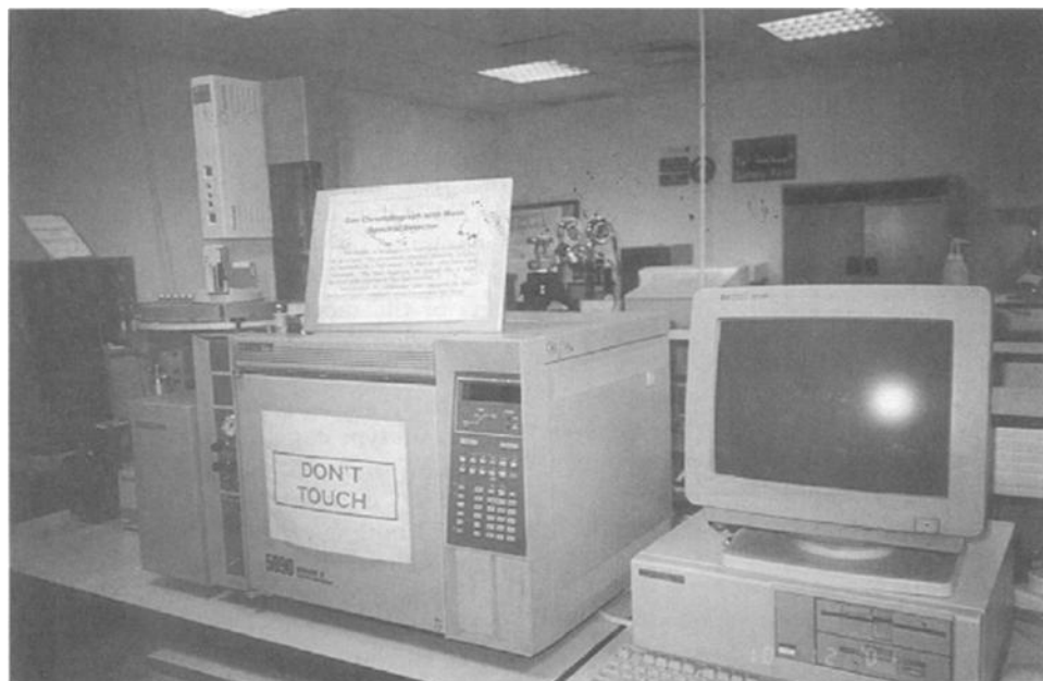
FIG. 3.16—HP made GC-MS model 5890 Series II. (courtesy of Chemical Engineering Department at Kuwait University).
