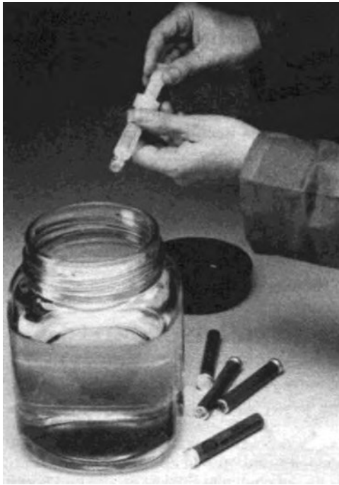
FIG. 1 A 5-mL syringe and detector capsule. (Reprinted courtesy of Shell International Trading Co., London, England.)
