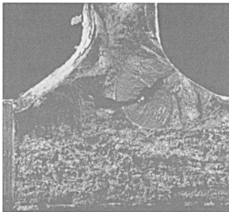
FIG. 7.18 Growth of a fatigue crack from irregularly shaped porosity maintaining a penny-shaped crack front.
