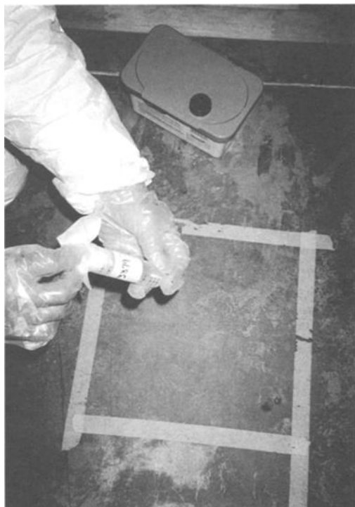
Figure 6.5: Collection of dust by wipe sampling
