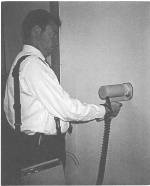
Figure 6.3: Photograph of X-ray Fluorescence (XRF) Paint Analyzer Being Used
