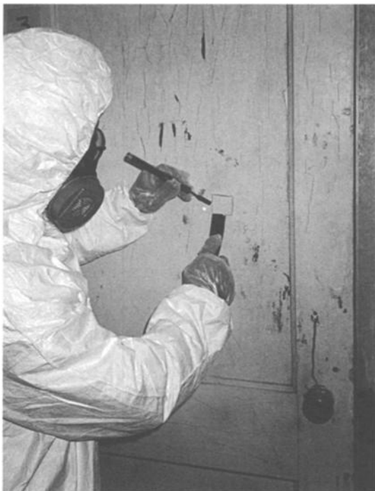
Figure 6.4: Collection of paint sample for laboratory analysis
