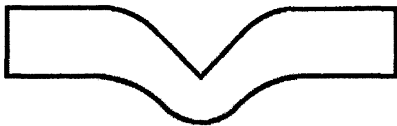
FIG. 3-10—“Die C” tear, ASTM D 1004.
