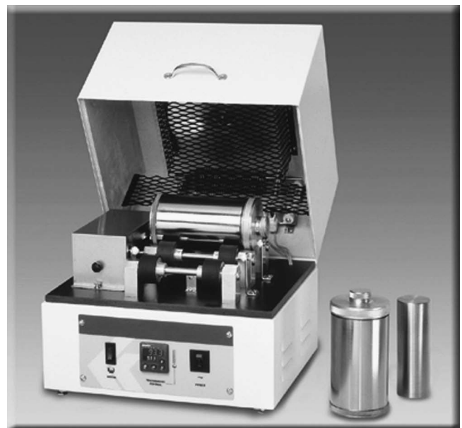
Fig. 5—Roll stability tester for ASTM D1831 (roll stability of lubricating grease).
