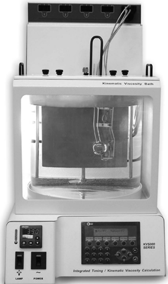
Fig. 10—Kinematic viscosity bath (ASTM D445).
