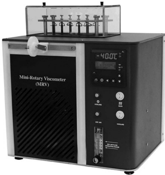
Fig. 14—Mini-Rotary Viscometer (ASTM D4684).
