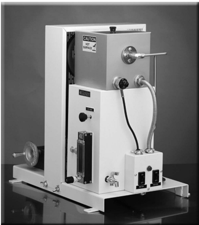
Fig. 20—EMCOR Grease Testing Machine (ASTM D6138).
