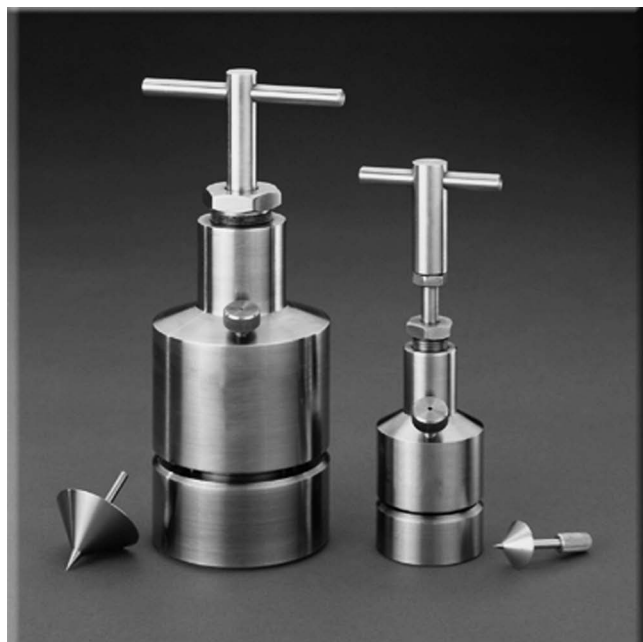
Fig. 3—One-quarter and one-half scale grease workers and cones (ASTM D1403).
