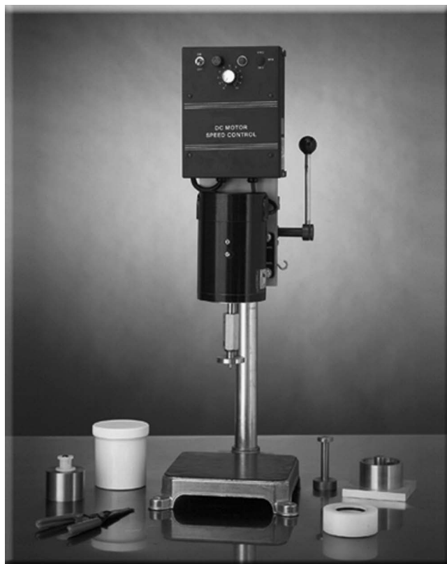
Fig. 19—Corrosion preventive properties apparatus (ASTM D1743).
