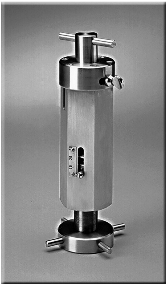
Fig. 22—Water spray apparatus (ASTM D4049).
