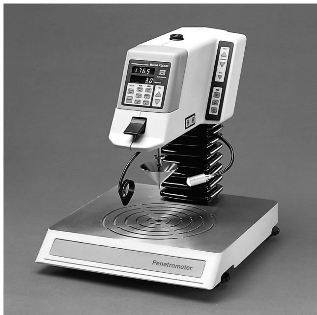
Fig. 2—Automatic penetrometer (ASTM D217).
