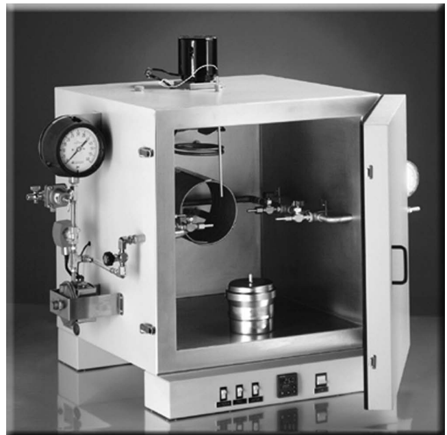
Fig. 12—Oil separation apparatus (ASTM D1742).
