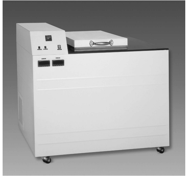
Fig. 7 —Test rig for ASTM D1478 to D4693 (low temperature torque tests).
