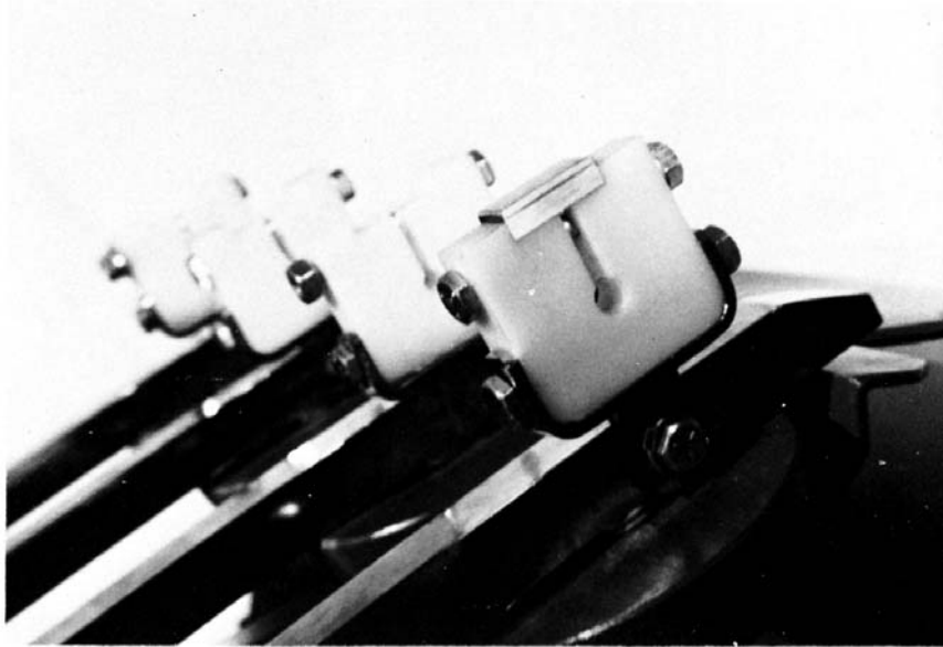
FIG. 5 Wear Block/Wear Specimen Holder
