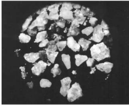
Bunker Hill Sand Miller Number 218
