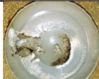
Partially-Ignited PA Valve Seat (post-test)
