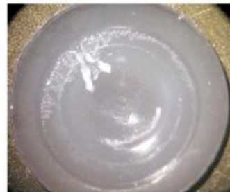
Partially-Melted PA Valve Seat (post-test)
