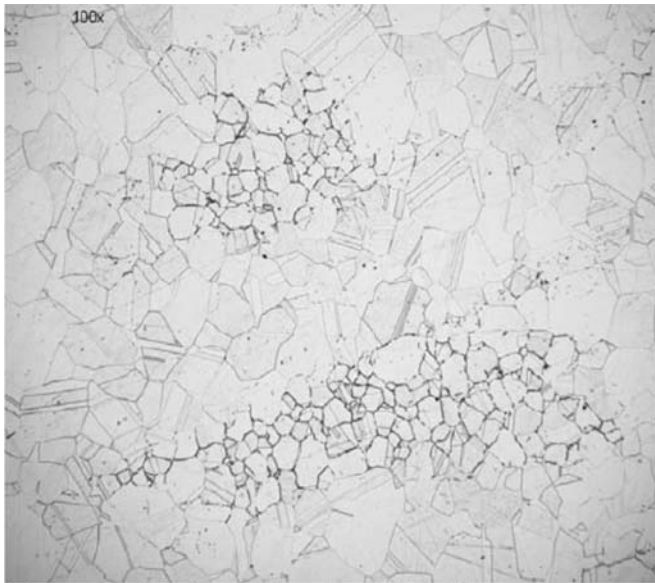
(a) 100X Original Magnification, Rejectable
