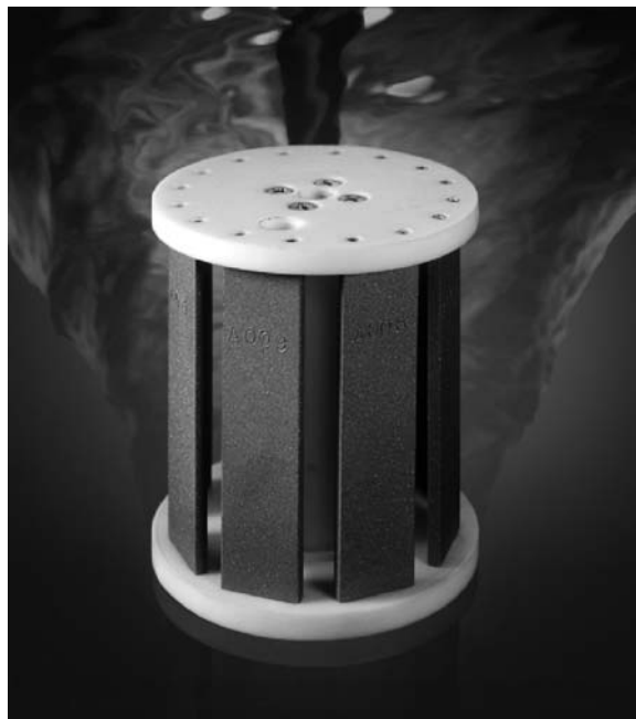
FIG. 2 Photo of Rotating Cage Containing Coupons
