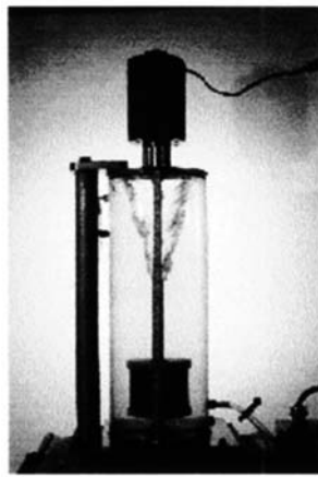
B. Top-cover Affected Zone (compare with A, the Vortex width decreases)
