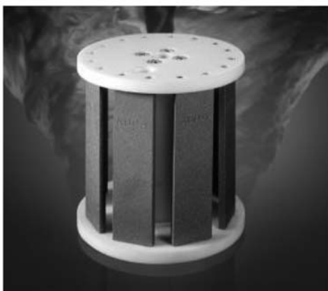
NOTE 1—The gap between the coupons (A) and the hole (B) introduce localized turbulence.
