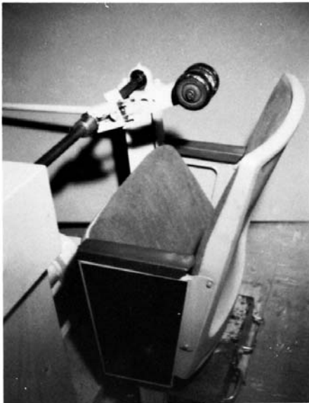
FIG. 2 Self-Rising Seat Mechanism Apparatus (Raised Position)
