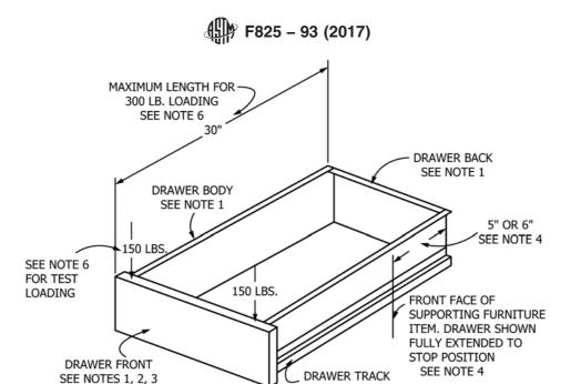
Note 1—Drawer front, body, and back shall be a minimum of 20 USSG (0.0359 in. or 0.91 mm) in accordance with Specification A366/A366M.
