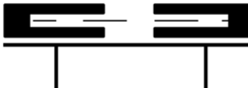
FIG. A1.7 Special Holder to Fit Exact Thickness of Specimen
