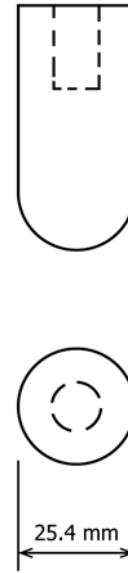
FIG. 3 Impactor Loading Nose—Type A Plate Specimen (Stainless Steel)
